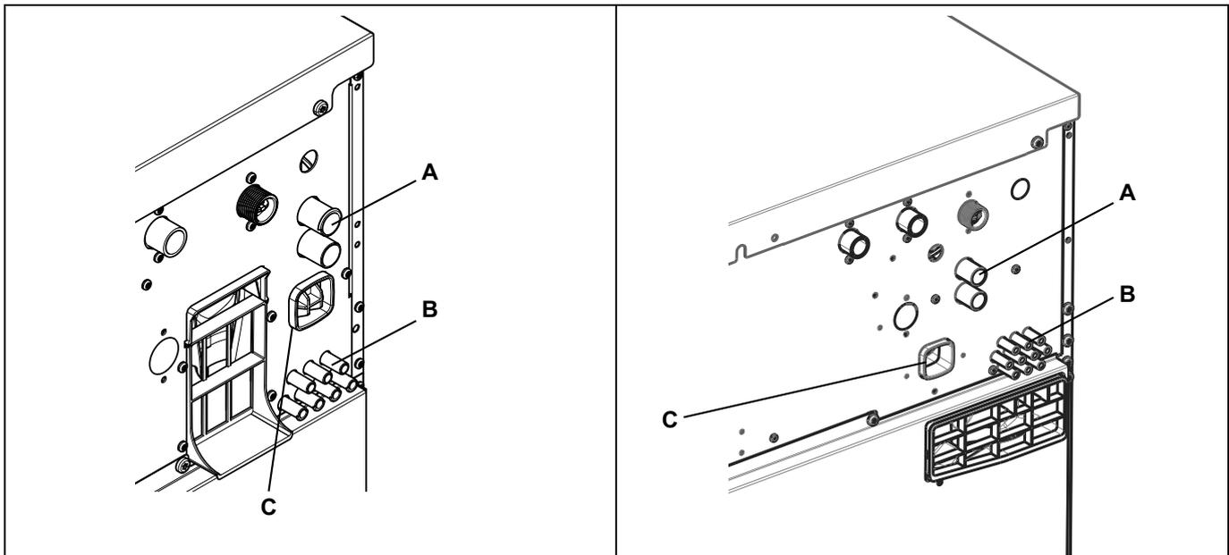
Always connect hoses on connections (A) with a hose clamp.
