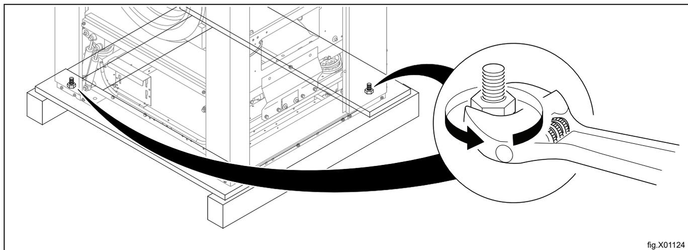
Remove the machine from the pallet.
