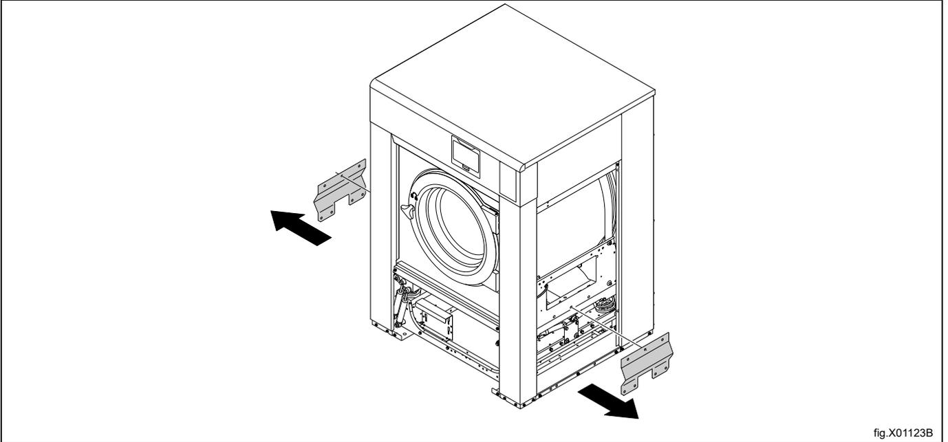
When the machine is placed in final position, mount the supporting feet. (If the machine is not to be mounted on a base).
